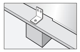
• Loosen the bracket that holds the appliance to the pallet.
